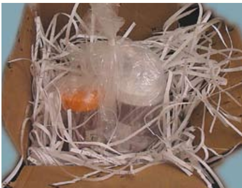
Plate 28: Brain specimens secured in screw cap plastic jar, sealed in two plastic bags, surrounded by sufficient absorbent material and packed in a firm cardboard box
